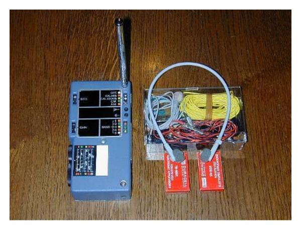
The Mark 328 was a solid-state miniature clandestine receiver developed by HMGCC at Hanslope Park (UK) c: 1970.
