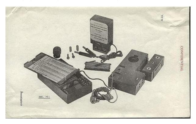
Developed towards the end of WW2 this miniature valved receiver was the more compact and reliable replacement for the MRC1.
